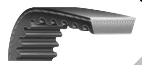
Synchronous belt with curvilinear tooth profile studied for transmitting elevated couple and power The optimized profile offers great resistance, a uniform distribution of the applied strengths and a redoubt noisiness. Good resistance to the commonly uses oils and temperatures among -25°C and + 100°C
