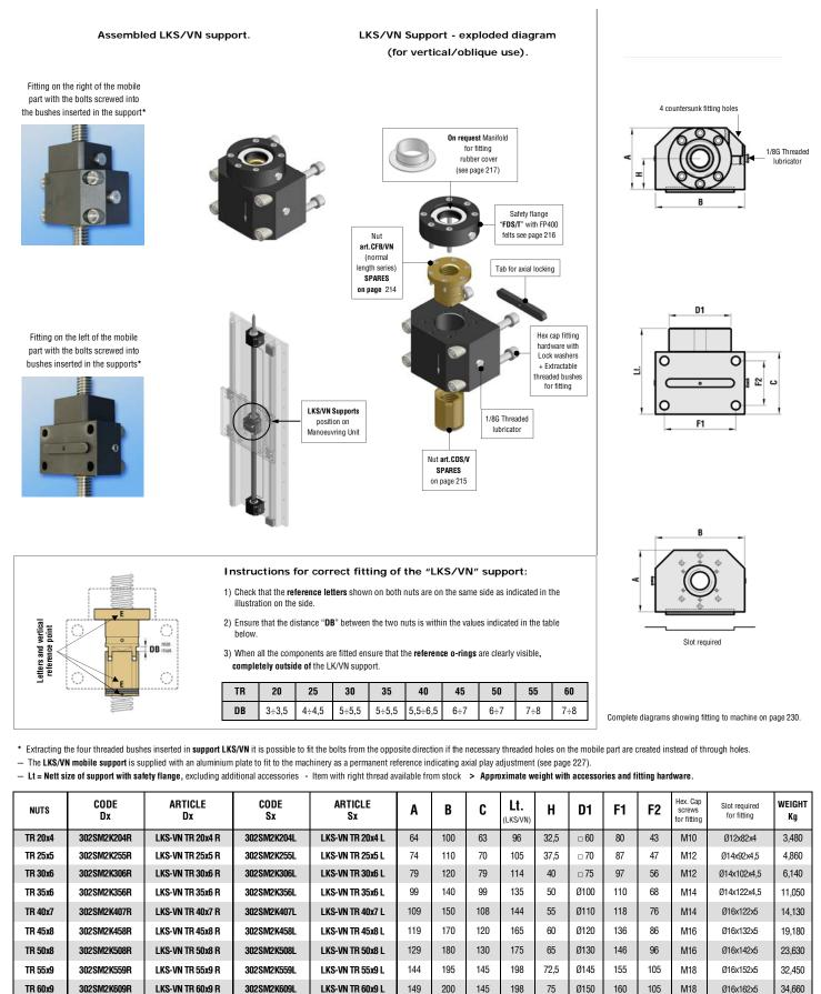
The supports above are shown assembled in the Tecnology KS/VN (Groups (see preceding pages) for which it is possible to calculate the total weight by adding them to the weight of the TR screw using the table on pag 182
