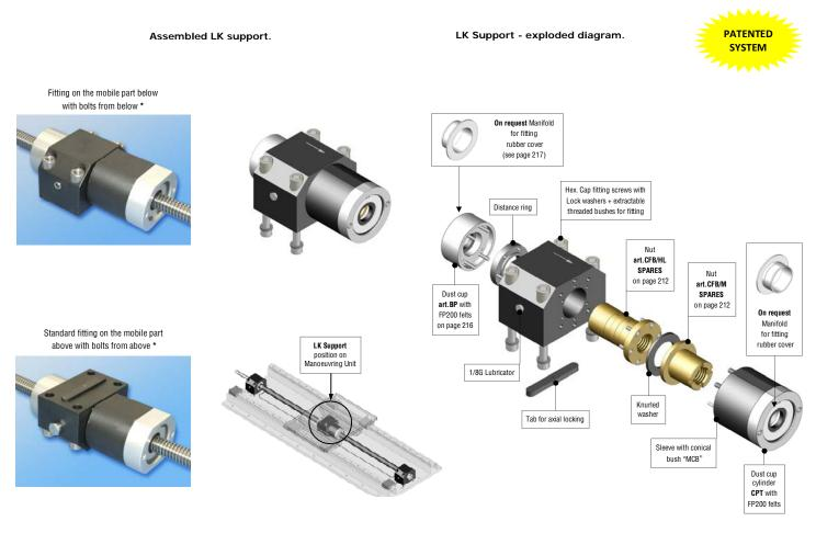
Extracting the four threaded bushes inserted in support LK it is possible to fit the bolts from the opposite direction if the necessary threaded holes on the mobile part are created instead of through holes.
