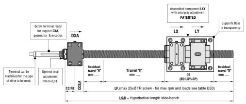
Lengths = D2 page 139 CCS/A page 148 CC/FB page 152 (normally the length D2 is substituted with the length of the entire carriage)
