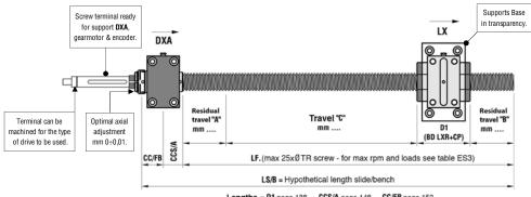
Lengths = D1 page 138 CCS/A page 148 CC/FB page 152 (normally the length D1 is substituted with the length of the entire carriage)
