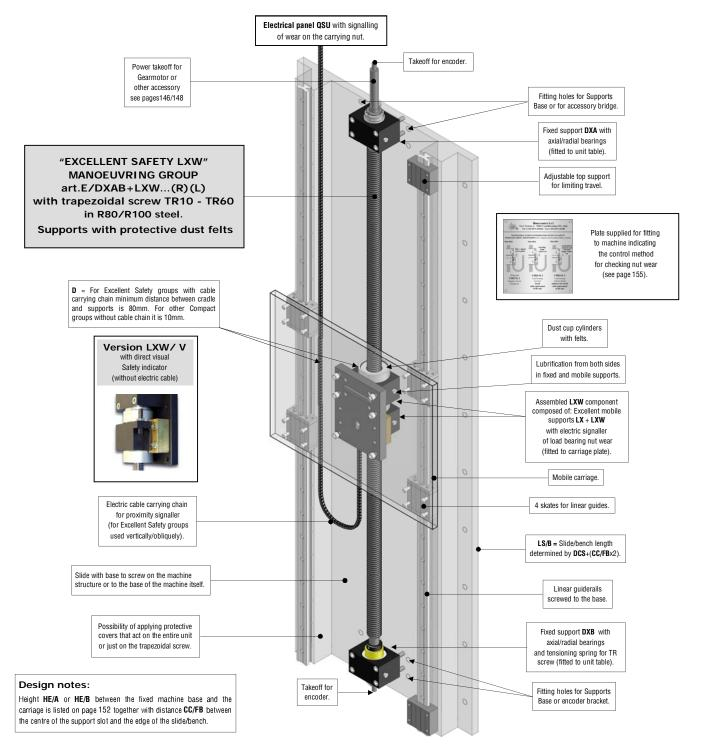
Group with right threaded components available from stock; with left threaded components made to order.
