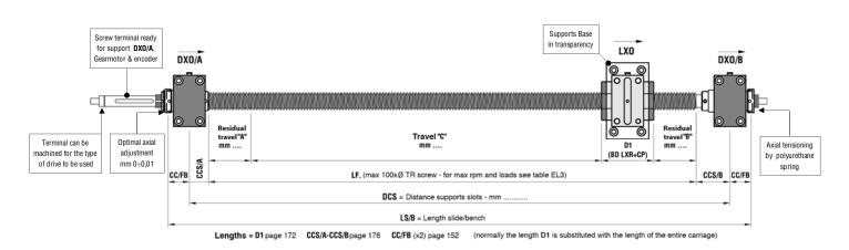
• TRAPEZOIDAL SCREW DESIGN of threaded bar ready for the above supports, gearmotor (positioned at the side or above) & encoder. For positioning the gearmotor below (for use only in cases of extreme necessity) please ask for the appropriate screw. Trapezoidal screw terminal: for specific details please see pages 146 - 148, for general details please see pages 48 - 56.
