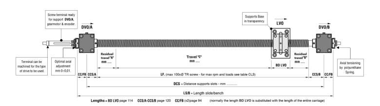
• TRAPEZOIDAL SCREW DESIGN of threaded bar ready for the above supports, gearmotor (positioned at the side or above) & encoder. For positioning the gearmotor below (for use only in cases of extreme necessity) please ask for the appropriate screw. Trapezoidal screw terminal: for specific details please see pages 88/90, for general details please see pages 48 - 56.
