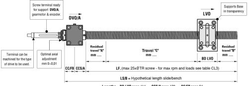
TRAPEZOIDAL SCREW DESIGN of threaded bar ready for the above supports, gearmotor (positioned at the side or above) & encoder.
