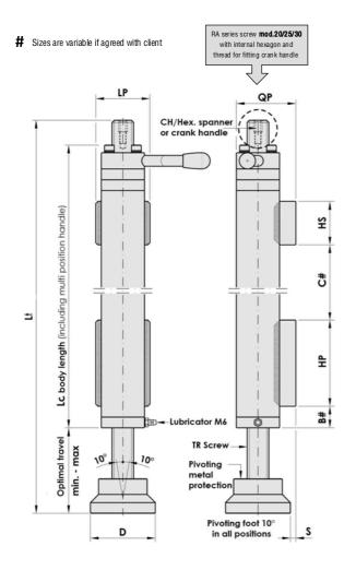
Illustration of a machine base using levelling Stabiliser. art.SLV...RA+ST740+PS mod.RA...F2 (article with fixed welded system, suitable for apply to machinery that need to be moved and repositioned frequently).
